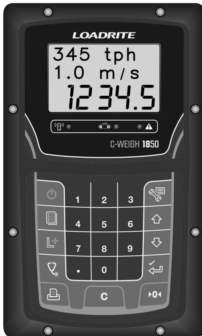
The display has internal memory, which stores settings and production data even when switched off.
