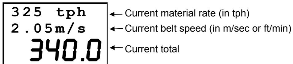
When the belt is running with load, the current total will count up. It is normal for the tph figure to change up and down (sometimes quite quickly) as material moves along the belt.
