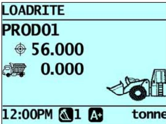
As you lift a weight, the target weight is displayed along with the current lifted weight and the potential weight if the lift is added.
